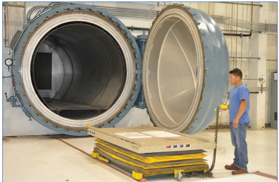
Jason Ford, 551st Commodities Maintenance Squadron aircraft mechanic, raises a KC-135 Stratotanker elevator skin panel to put in the autoclave for metal-to-metal bonding. Similar to an oven baking cookies, the autoclave cures composites under nitrogen pressure and electric heat. Autoclaves are energy hogs and to help keep costs down, workers monitor their usage but are careful not to impact production. (U.S. Air Force photo/Brandice J. O'Brien)
