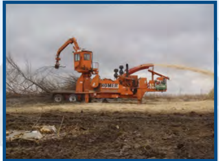
Whole tree chippers mulched all trees and brush onsite eliminating burning or removal of brush from the site.
