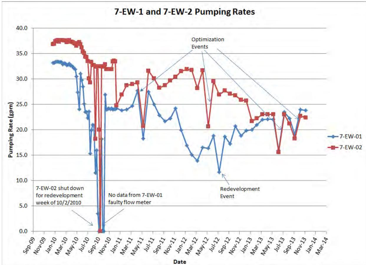
Extraction well 7-EW-1 was redeveloped in July of 2008 following a sharp decline in the sustainable pumping rate. Following redevelopment, the flow rate for 7-EW-1 remained relatively stable through 2011 but began declining again in 2012. 7-EW-1 was redeveloped in July 2012, and the flow rate increased to approximately 21 gpm.
