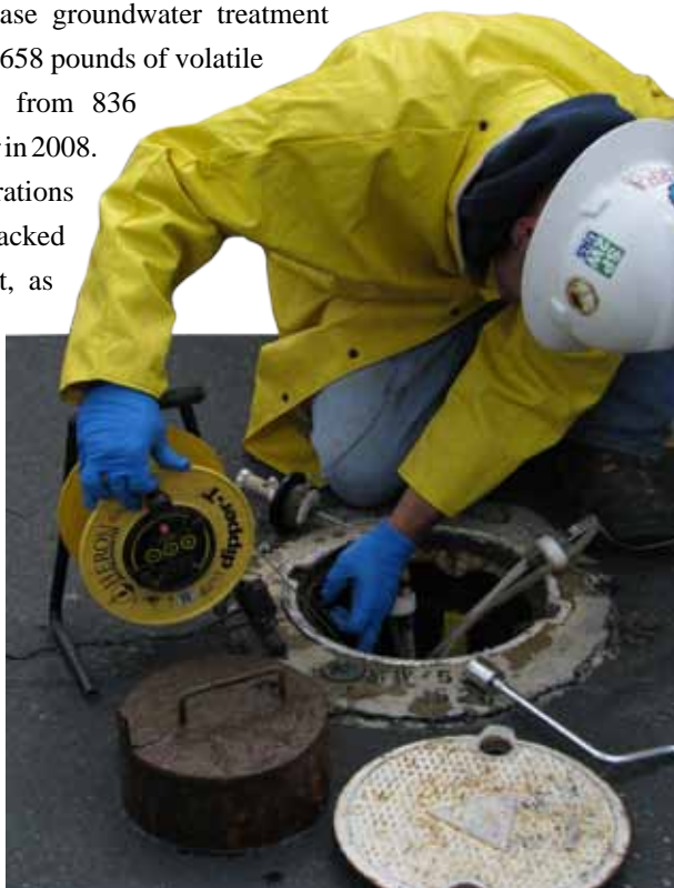
Field technicians monitor groundwater levels and contaminants throughout the year to track the flow and concentrations of contaminants.
