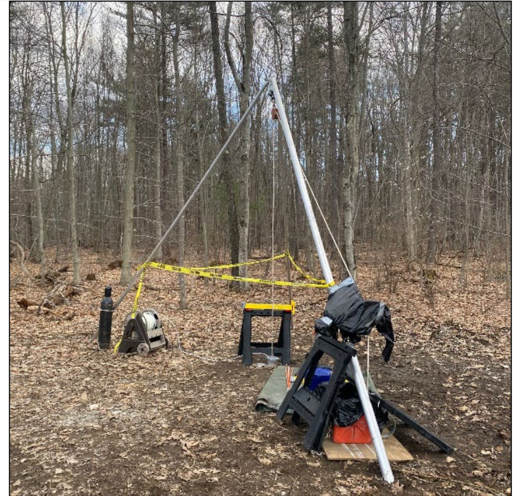
Top: A packer sampling set up.
