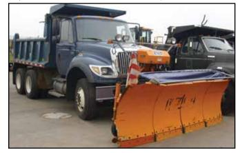
(above) Dump trucks equipped with snowplows are used mainly for street-side snow clearing. (U.S. Air Force photo/Preston "Benny" Benedyk/Released)
