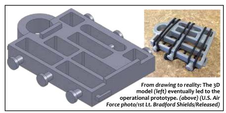
removing each sensor from the robot. Although this is an effective, low-cost solution, it takes a significant amount of time to change sensors in the field and during post-mission clean-up. A universal bracket would reduce that time and effort, but no bracket capable of mounting differently shaped sensors to the UGV is commercially available.
