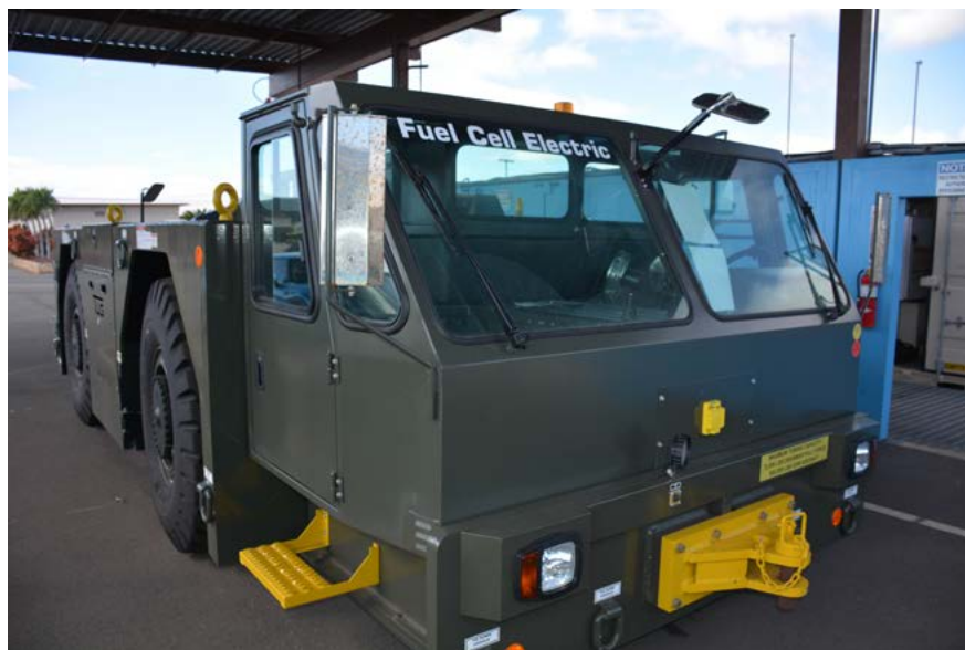
This U-30 heavy aircraft tug is powered by a hydrogen fuel cell. This vehicle is part of a demonstration of hydrogen as an alternative fuel source at Joint Base Pearl Harbor-Hickam, Hawaii. (U.S. Air Force photo by J. Brian Garmon)
