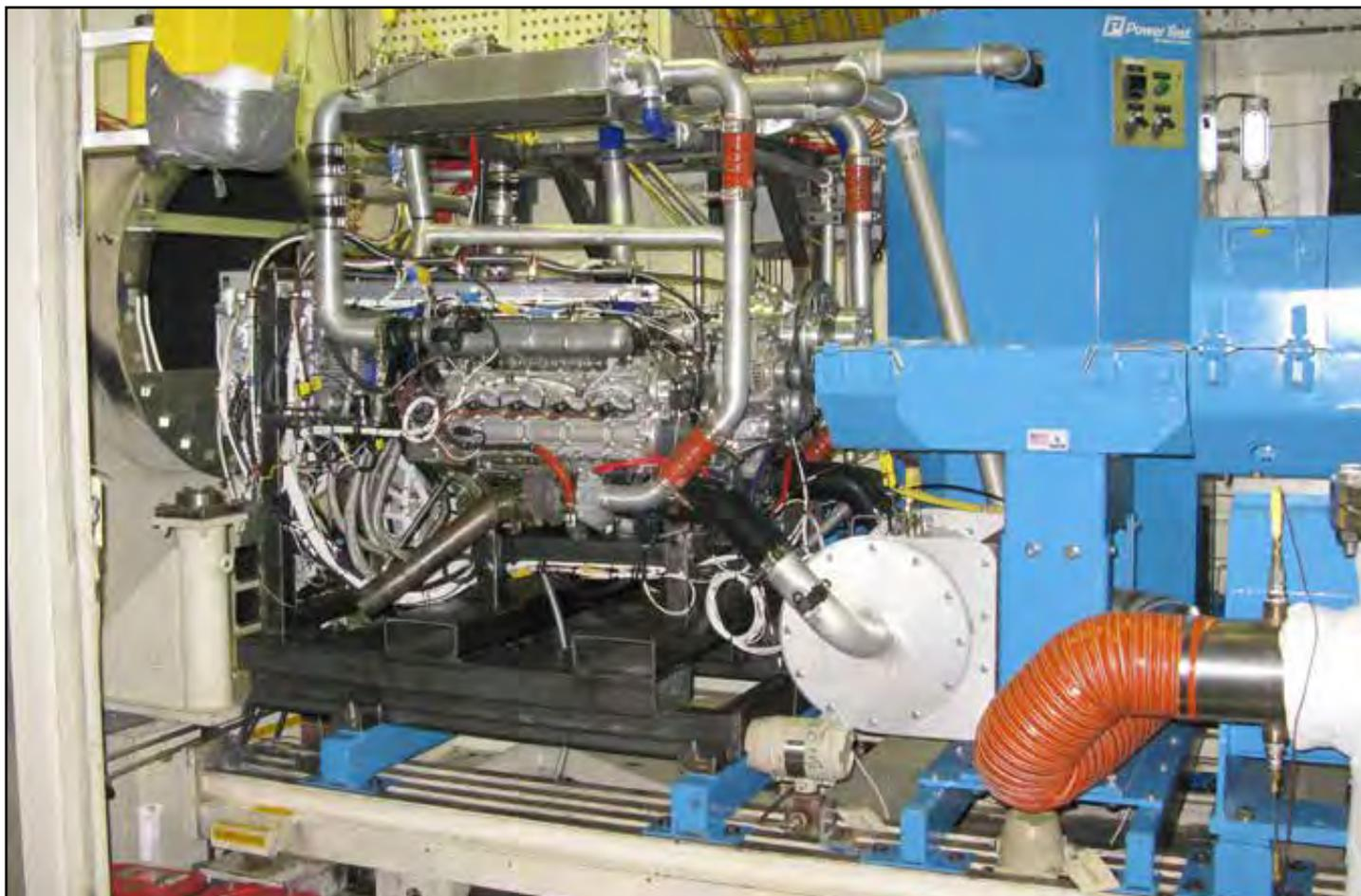
The Air Force Research Laboratory Advanced Power Technology Office's high efficiency innovative aviation diesel engine is shown here in the Arnold Engineering Development Center T-11 Test Cell. The Graflight engine, developed by Engineered Propulsion Systems, could offer extended range and greater fuel options for unmanned aircraft missions. (Courtesy photo by AEDC)
