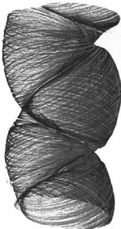
Scientists at the Air Force Research Laboratory are exploring the use of carbon nanotube-based twistron yarns for energy generation. This twistron yarn image, captured by X-Ray tomography, is a 3-D rendering of the coiled nanotube fibers. (U.S. Air Force photo by Matt Lucas)
