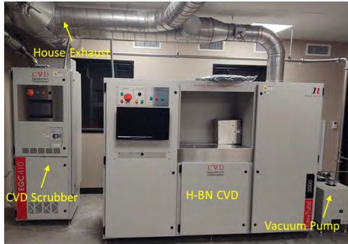
EasyTube® 3000 – H-BN Chemical Vapor Deposition System
