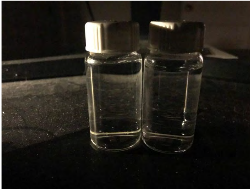
Water samples under subdued light after aeration by MNBA (left) and before aeration (right), showing no differences in appearance.
