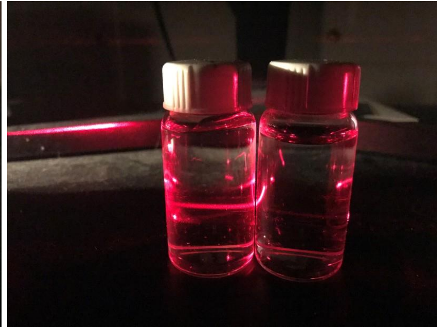
Water samples illuminated by a laser pointer after aeration (left) and before aeration (right), showing strong scattering of the laser beam by nanobubbles created by aeration.
